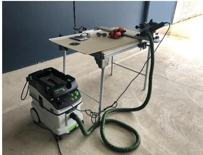
The external sampling setup for sample M3288/3. The Diamond Cutting angle grinder system is seen attached to the extractor with no -pre-separator attached.
