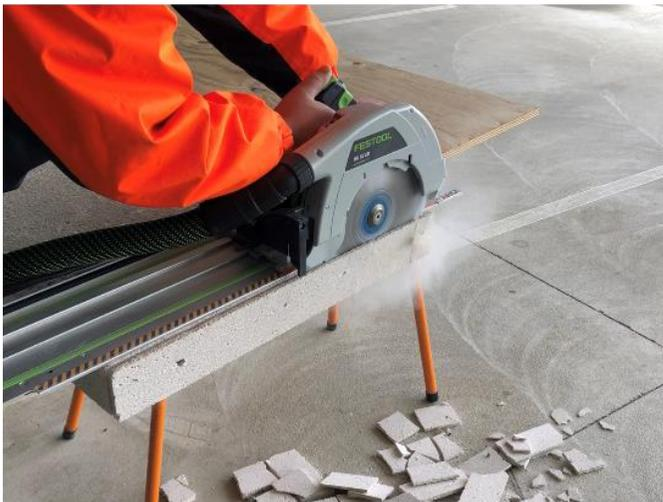
The HK 85EB circular saw cutting the Hebel product (Sample no. M3288/2). This was the only sample to return detectable results for RCS and also produce the highest total respirable dust results.
