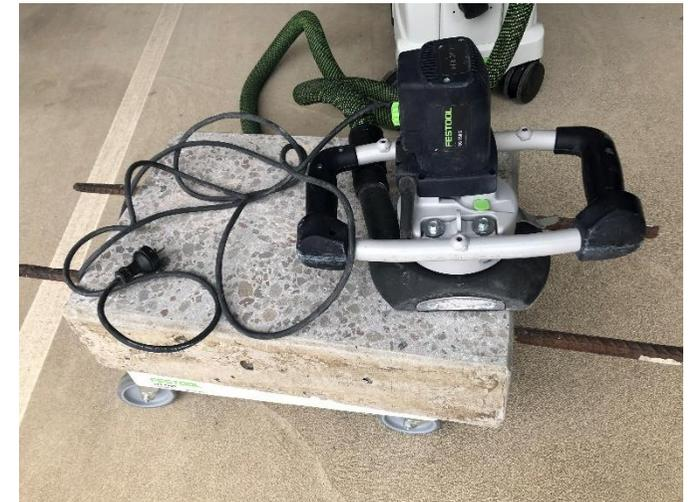
The Festool RG 150 E grinder used to grind concrete in sample M3288/5. Results from this sample were well below the relevant exposure standards.
