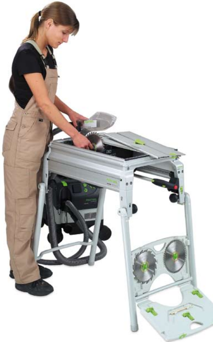
2 Easy access to the blade: the retaining flap is unlocked using the rotary knob; the spindle stop locks into place automatically.
