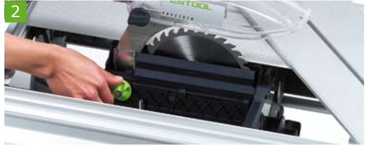
2 Easy access to the blade: the retaining flap is unlocked using the rotary knob; the spindle stop locks into place automatically.
