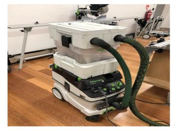
The CTM 36 AutoClean Dust Extractor with the pre-separator cyclone unit attached. This extraction setup was used in samples M3288/1,2,5 and 6.
