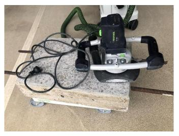
The *Festool* RG 150 E grinder used to grind concrete in sample M3288/5. Results from this sample were well below the relevant exposure standards.
