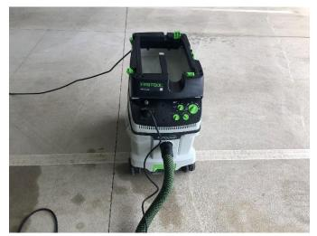
The CTM 36 AutoClean Dust Extractor with the pre-separator unit not attached. This extraction setup was used in samples M3288/3 and 4.
