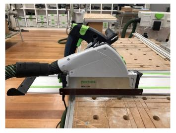
The *Festool* TS 55 Plunge Cut saw with dust guard. This unit was used in samples M3288/1 and 6.
