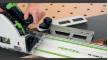
2 Combination bevel: for direct transfer of angle to workpiece.
