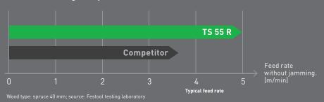
Dutstanding feed rates: up to 5 m per minute without jamming. MMC-Electronic keeps the speed at a constant level, which you can set as required. Soft start, protection from overheating and overloading and triple motor bearings provide durability, while the quick-acting brake provides safety.
