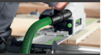
4 Deflector: helps the dust extraction hose to slide perfectly.
