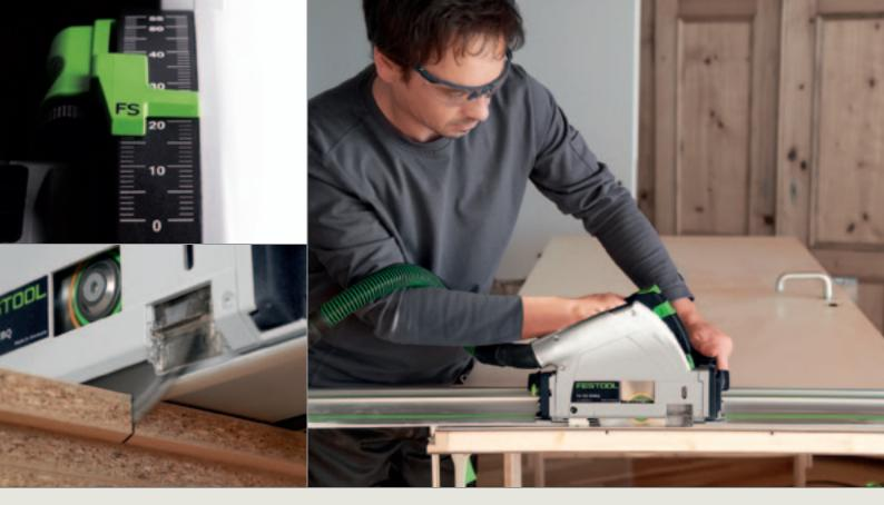
Easy to read and to set: the dual cutting depth scale for work with and without a guide rail. With extra-large print and the option of fine adjustment. For top-quality results work with the guide rail for clean cuts, free of tear-out. The TS 55 R is secured with guidance jaws, which are adjusted without the need for tools, for zero-play motion along the rail.
