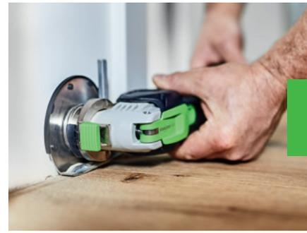
**Quick-clamp system with StarlockMax tool adapter**
