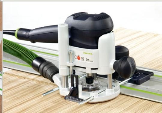
Vital for furniture building – router and guide rail with positioning holes make for easy work on shelving systems or fittings.
