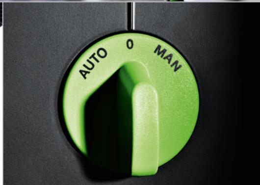
The choice is yours – with the switch in the “MAN” position, dust extraction is started manually when the EAA is switched on. In “AUTO” position, it starts when the power tool is switched on. And in “0” position all that is activated is the power supply via the socket with continuous power.
