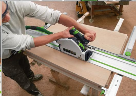
Simply precise – the width of the workpiece can be conveniently adjusted using the parallel side fence with scale and adjustable stop.
