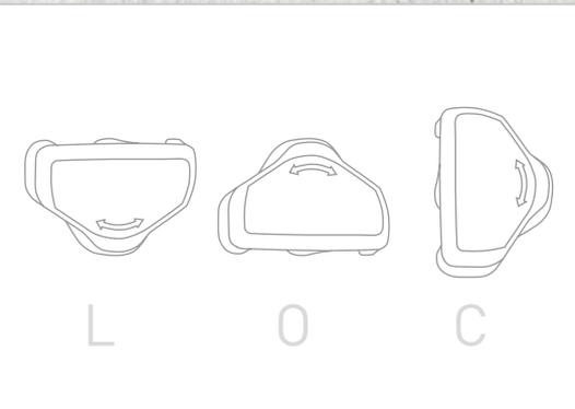
Three functions combined – the central control element of the T-LOC SYSTAINER. Lock, open, connect with just one turn of the latch.
