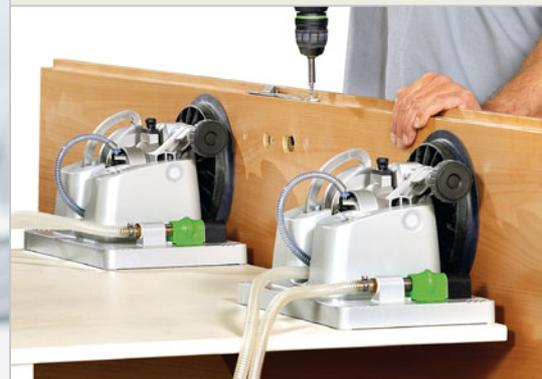
Work on pieces from all sides – they can be rotated through 360° and pivoted up to 90°. So you can work ergonomically without re-clamping.
