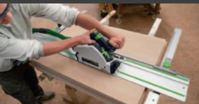
5 Parallel side fence: ideal for low-volume batches of identical cuts.
