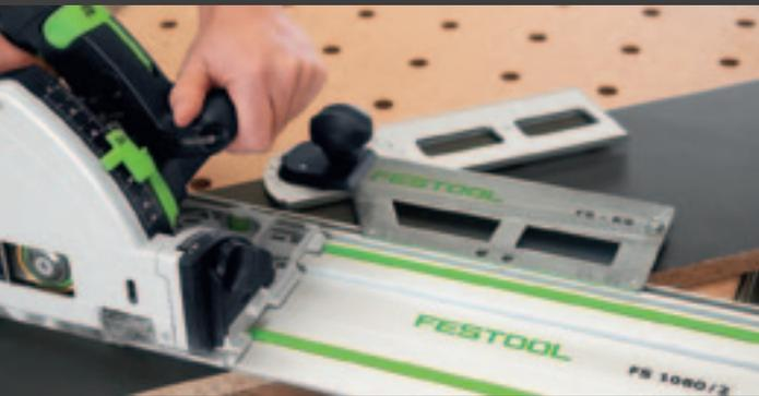
2 Combination bevel: for direct transfer of angle to workpiece.
