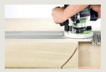
You can also save yourself a lot of time-consuming effort in making templates for large radius cuts whose centre points extend beyond the workpiece - just use the extension profile for the MFS routing template. The centring pin is attached to a suitable base outside the panel to be cut and the router, with a suitable bit, is positioned in the copy ring holder. The result is accurate to the millimetre, even for very large radius cuts.
