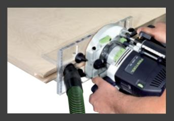
Preparing solid wood doors for weatherstip inlays is generally a job done in the workshop on a spindle molder. With Festool routers and accessories, this type of work can be performed on site with identical results. Add in integrated dust extraction and the site remains free of dust while the work is being performed.
