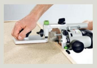
With Festool's innovative routing accessories, solid edging up to 28 mm thick can be trimmed with the handy OF 1010 router. By using the fine settings, precision in 1/10 mm increments is possible. Preparing edging is accomplished quickly and accurately, which is especially important for custom work.
