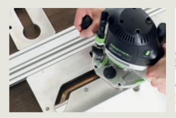
It is difficult to join rounded off or profiled wood panels at  $90^{\circ}$  angles. It is easier to use the APS benchtop template because clean edge joints are then guaranteed. The template allows precise results – even for repeated cutting in the same trench. The routing template can be re-positioned on the surface so that benchtops of up to 900 mm wide can be joined.
