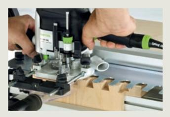
Cutting dovetails can be painstaking manual work. Or it can be done quickly and easily by using the VS 600 joining system. Because here, the router, template and copying ring are perfectly  $matched \ to \ each \ other \ so \ that \ precise \ results \ can \ be \ produced.$
