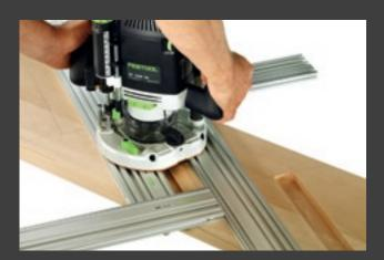
When cutting stair stringers, the slope and tread dimensions usually have to be re-measured and laid out again and again. Using the Festool routing template, you simply set up the trench angle and tread dimensions once, then slide it along the stringer to the next tread position. It's far easier and more efficient than traditional layout methods.
