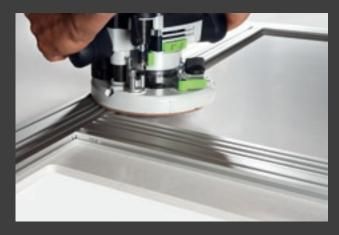
Cut-outs must be precise, especially when trenching in stages through thick panels. The routing template provides the precision - it can be set to the proper dimensions, fastened down and then you can rout through the material in one or more exactly identical stages. The shapes will match perfectly.
