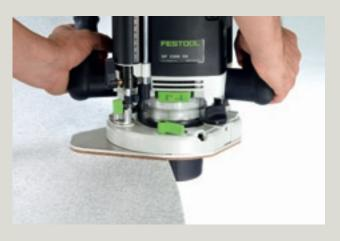
When routing edges, the balance of the router using a normal base is not ideal. It can tilt at any time and ruin the edge. Using the wide base from Festool, the support area is increased and the secure guidance of the router guaranteed. In seconds and without tools, you can replace the standard base with the wide base.
