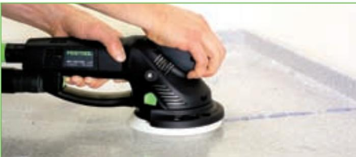
For removing dried excess adhesive from mineral surfaces.
