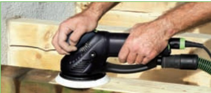
For coarse sanding of weathered beams.
