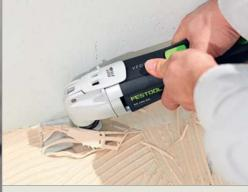
The scraper makes it easy: removing adhesive residue or silicone.
