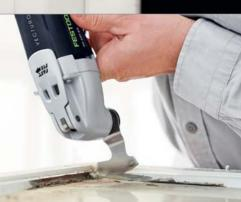
The special blade for window installation for removing putty from window panes.
