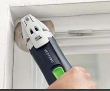
Right up to the edge: with the saw blade with depressed centre.
