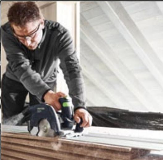
**Precision guidance:** The HKC 55 demonstrates its versatility when combined with the Festool guide rail system, too. So, for example, insulation boards can be cut to size quickly and accurately using the FS 1400/2.
