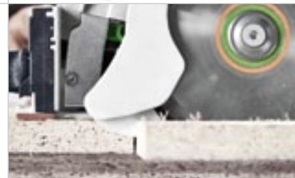
**Viewing window and cutting indicator:** The open construction and the viewing window on the inside provide a good view of the scribe mark and saw blade. The continuous cutting indicator also increases precision.
