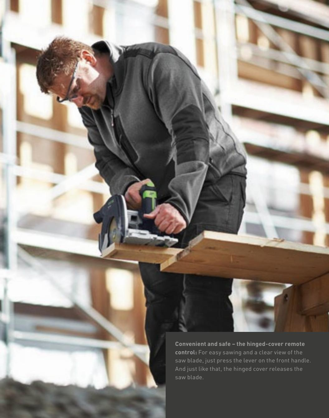
**Convenient and safe – the hinged-cover remote control:** For easy sawing and a clear view of the saw blade, just press the lever on the front handle. And just like that, the hinged cover releases the saw blade.
