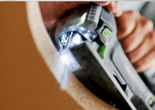
Accurate sawing along a scribe mark – the strobe light makes the blade seem to stand still, while dust extraction and the blower function of the CARVEX give you a clear view of the scribe mark.
