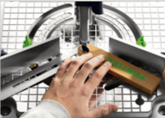
Couldn't be easier – use the bevel to record the angle from the wall or recess, transfer it to the stop system and make the cut.
