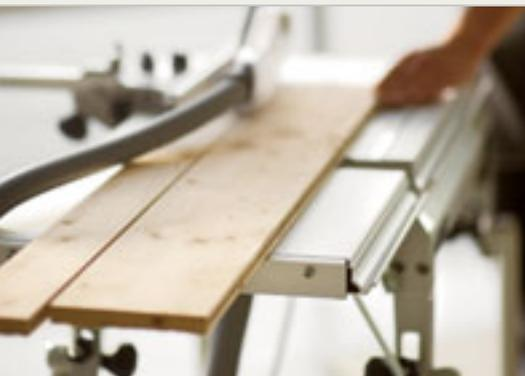
Easily expanded – the extension table allows rip cuts on large workpieces.
