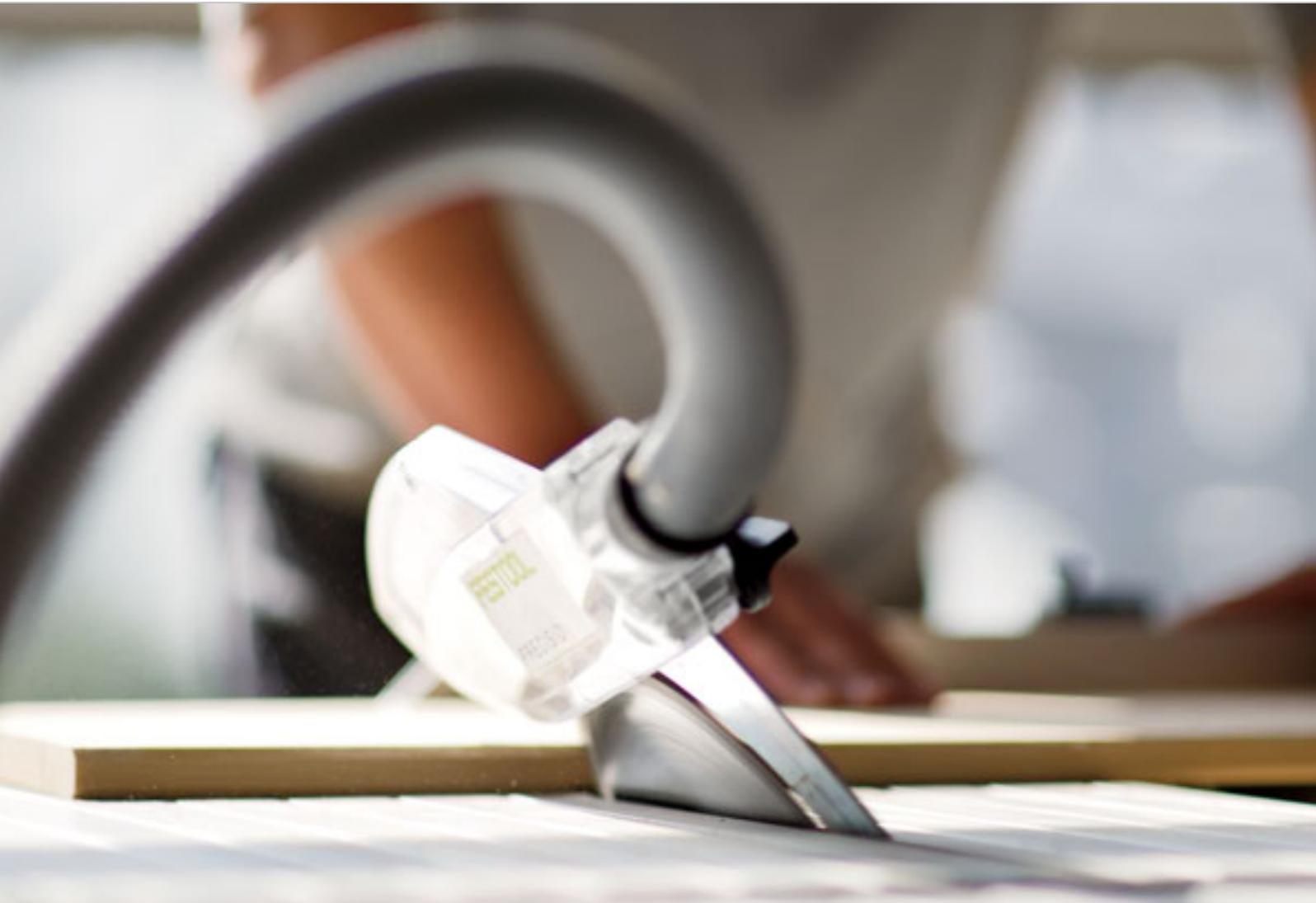
Always accurate – the pivoting blade allows precise angled cuts from  $-2^{\circ}$  to  $47^{\circ}$  or rip cuts up to a cutting height of 52 mm (CS 50) or 70 mm (CS 70).
