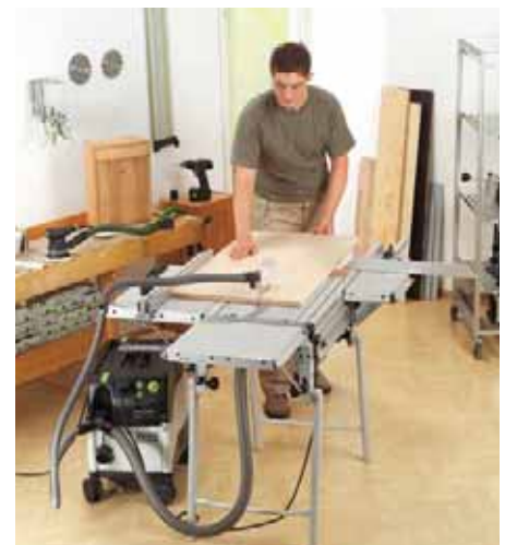
Once the module is inserted into the basic unit, you can start working. The hand-held machine has been converted to a bench-mounted system.
