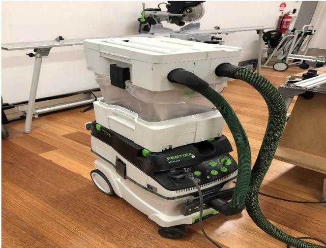
The CTM 36 AutoClean Dust Extractor with the pre-separator cyclone unit attached. This extraction setup was used in samples M3288/1,2,5 and 6.
