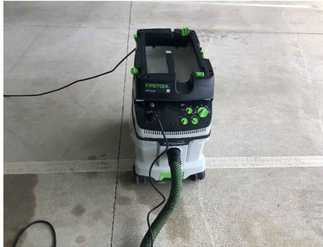
The CTM 36 AutoClean Dust Extractor with the pre-separator unit not attached. This extraction setup was used in samples M3288/3 and 4.
