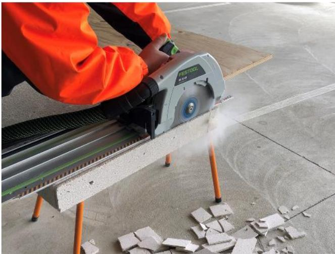
The HK 85EB circular saw cutting the Hebel product (Sample no. M3288/2). This was the only sample to return detectable results for RCS and also produce the highest total respirable dust results.
