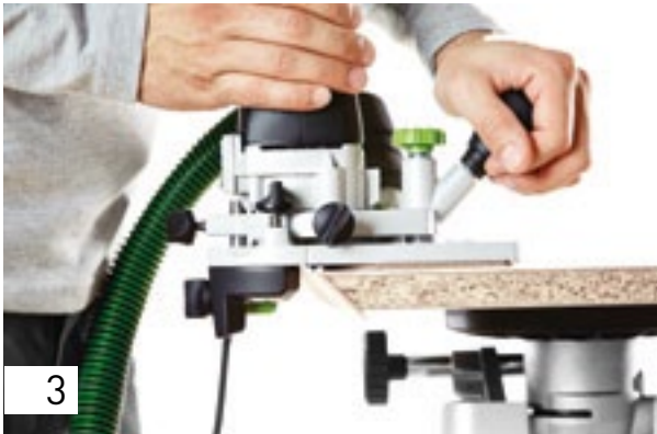
3 Make sure that the extraction hood under the machine is resting directly against the workpiece as this can be used as a guide. Then create the radius on the wooden edge using sandpaper.
