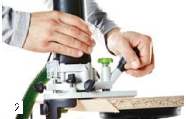
2 Then mill the workpiece flush.
