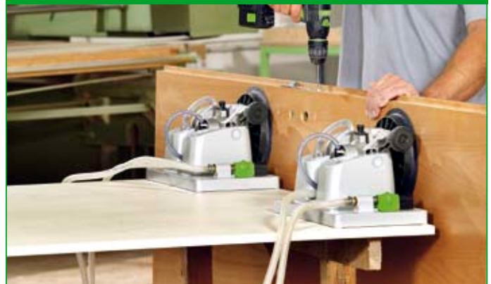
Clamp larger, heavier workpieces
