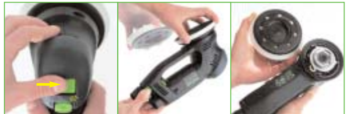
Set the switch on the ROTEX® Press the spindle stop and turn to rotary motion. Press the spindle stop and turn the pad anticlockwise. Put on a new pad and turn to secure.
