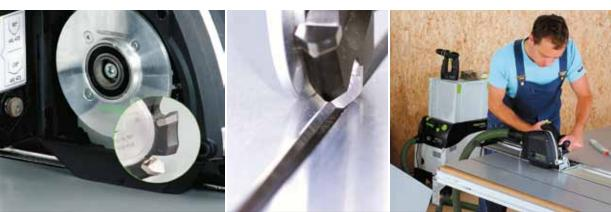
Fast, Precise Bends in Aluminium Composite Materials on Site
