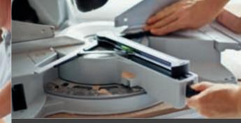
Dual-line laser and bevel for precision indication of the cutting line and angle transfer.
