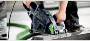
The plunge cut function allows you to start cutting at any point on the workpiece.
