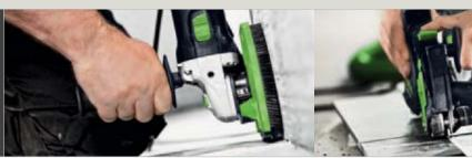
Guide rail for precision: the cutting system can be used in combination with the Festool guide rail for a precise cut.
