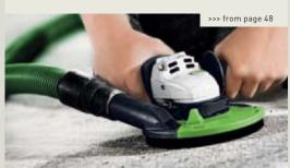
DSC-AG 125: Diamond cutting system. Ideal for virtually dust-free cutting to depths of 27 mm.
