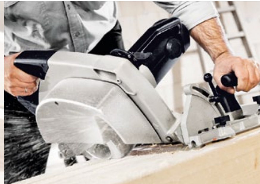
Saw blade off, bird's mouth bit on: The HK 132 E circular saw can be turned into a reliable bird's mouth router with little effort using the bird's mouth attachment.
