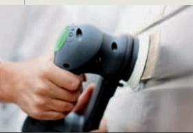
Quick results in a single step: the new 90 mm pad was developed specifically for window frames and tongue and groove joints.
