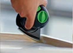
Save on costs: the tips of the sanding pad and abrasive can be used three times simply by rotating.
