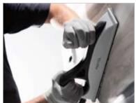
8. After complete drying of the filler apply guide control black (see Fig. 523/19 and 523/22) and use the hand sanding block and sanding discs Granat P280 to surface grind the last irregularities (see Fig. 523/24)
